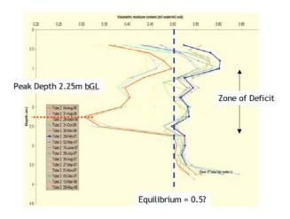
Above are the general characteristics of the profiles. This is the plot of NP 2 (just outside the canopy and nearest to the 'drip line') which shows the widest seasonal fluctuations with the soil rehydrating completely, recovering in one season.
