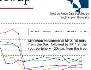
Tim Freeman kindly provided a method of estimating water uptake based on volumetric measure. By multiplying the soil/root volume by the change in volumetric moisture we can estimate the water uptake. Our average 7.3% moisture deficit in  $\pi \times 25^2 \times 1.2$ m average volume of soil = 0.073 x 2,355m<sup>3</sup> = 172 m<sup>3</sup> - 172,000 ltrs in a year.
