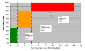
He proposes a simple set of rules whereby if movement of 'x'mm has taken place, then 'y' happens. In extreme cases that might lead to underpinning or tree removal, but in other instances, the tree would be retained and the property repaired.
